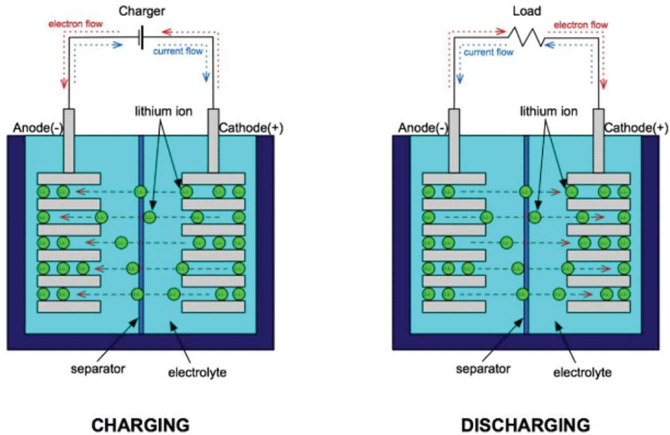
**Figure 1: Lithium-Ion Battery**
